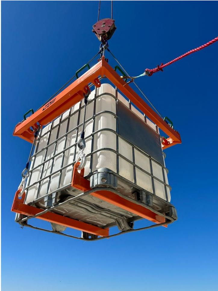
**IBC Lifting with Pallet Bars**
