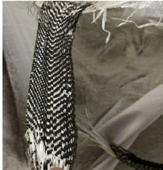
Figure 2: Failed Lifting Point
