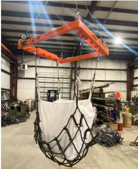
FIBC Lifted with IBC “Spacer” Slings
