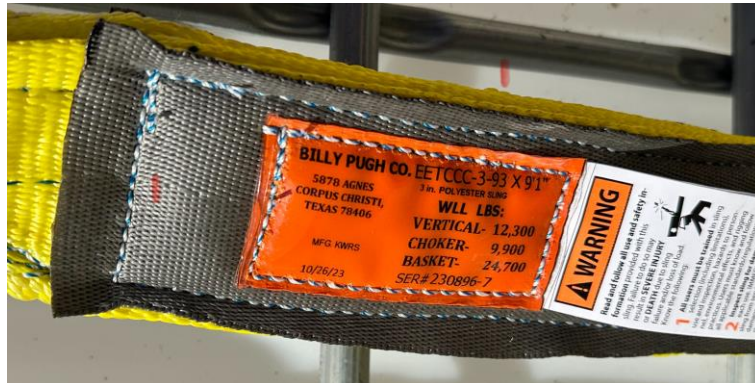
3", 3-Ply Polyester Sling with a 12,300 lbs Capacity in Basket Configuration
