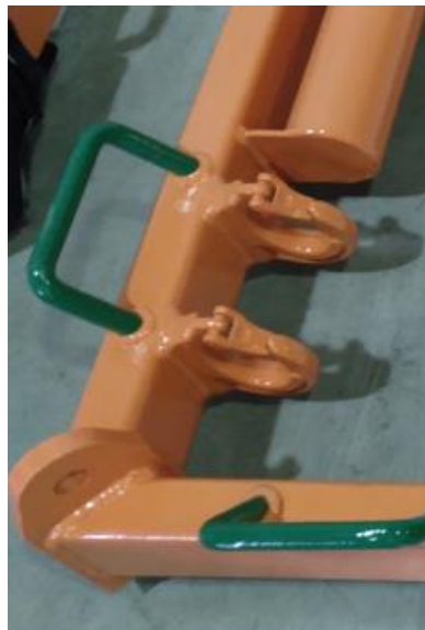
Radiused Internal Bumper and Hook “Pocket”
