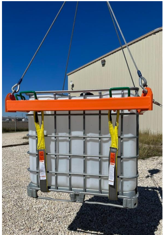
Lifting IBC Tote with Soft Straps
