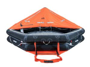
Upon release from its stowage arrangement, this type of liferaft either slides automatically or is thrown overboard manually. Once waterborne, the liferaft inflates by a firm pull to the painter line.
