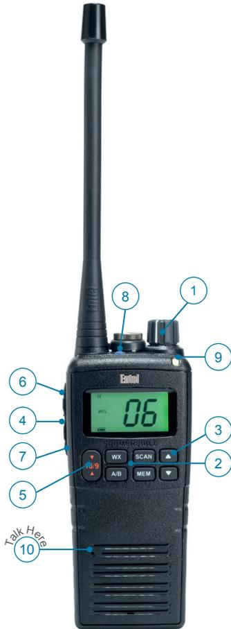
1. On/off knob. Rotate to turn the radio on or off, rotate clockwise to increase volume
